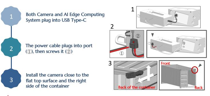
\* Put the AI Edge Computing System in front of the camera in case of covering the viewing angle
